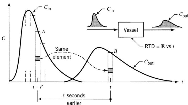
Figure 11.15 Sketch showing derivation of the convolution integral.
