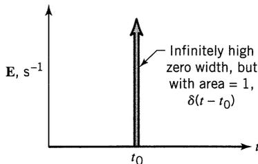
**Figure 11.18** The  $E$  function for plug flow.
