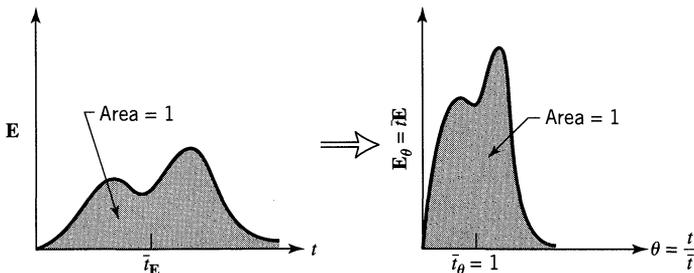
**Figure 11.10** Transforming an  $\mathbf{E}$  curve into an  $\mathbf{E}_\theta$  curve.
