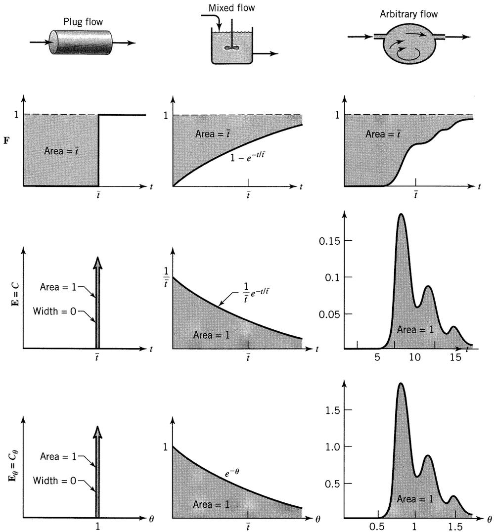
**Figure 11.14** Properties of the  $E$  and  $F$  curves for various flows. Curves are drawn in terms of ordinary and dimensionless time units. Relationship between curves is given by Eqs. 7 and 8.
