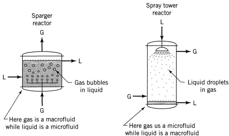
**Figure 11.3** Examples of macro- and microfluid behavior.
