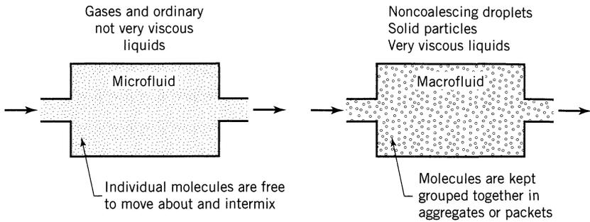
**Figure 11.2** Two extremes of aggregation of fluid.
